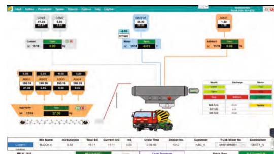
Control System & AQ-SMART Software
